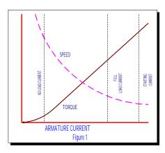
As shown in the typical performance curves of Figure 1, the high torque at low speed characteristic of the series motor is evident.
